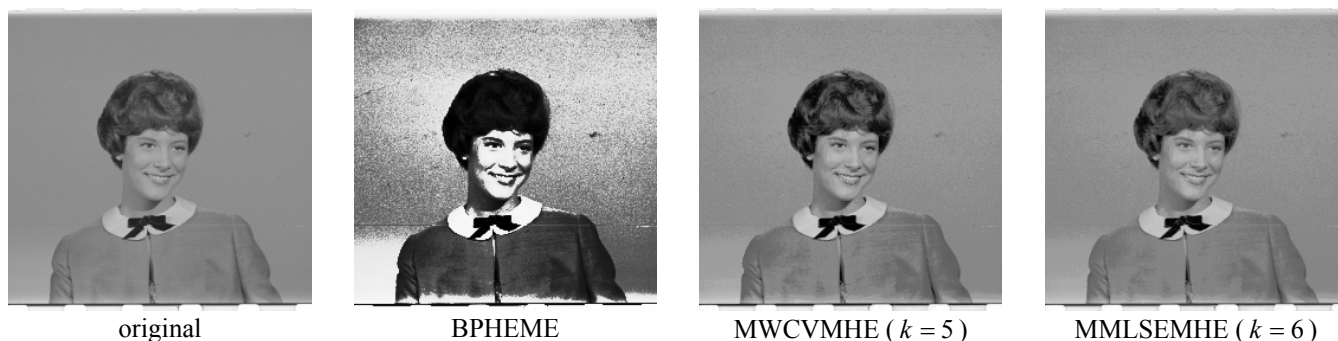
Fig. 2. Enhancement for the girl image based on BPHEME, MWCVMHE, and MMLSEMHE methods.
